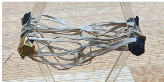
Figure 4.1.1: Rubber bands knotted together to extend their operating length and vary the phase of their engagements stored energy during the loading phase of the jump.
