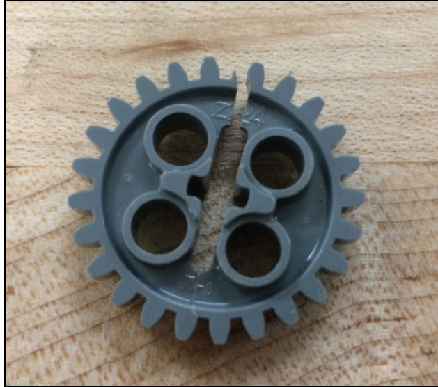
Fig. 5.5.1: The most failure-prone gear in our transmission
